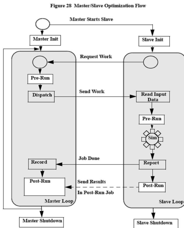
Figure 1 The master/slave structure used by Trick's optimization method [1]
