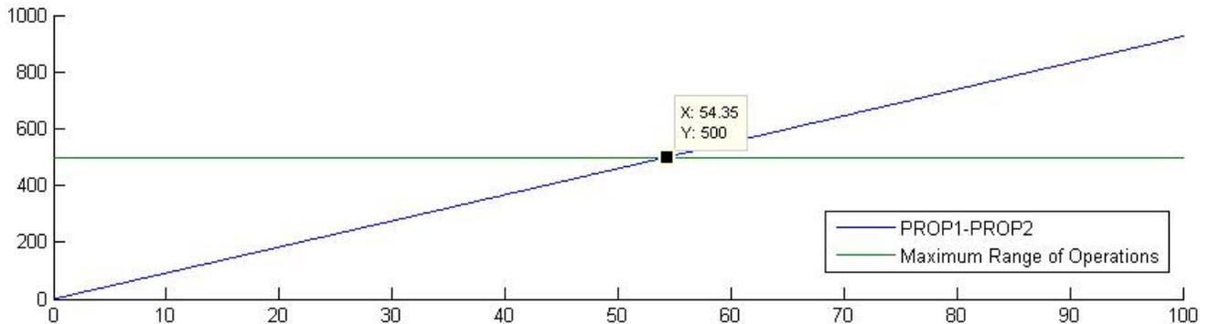
Figure 5: Relative Distance between CubeSats (km) as a function of Time (solar days)
