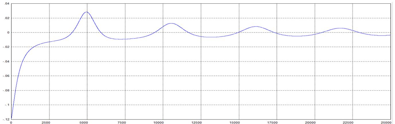
Figure 8: Angular Rate requirements (deg/s) for PROP1 over first 25000 seconds.
