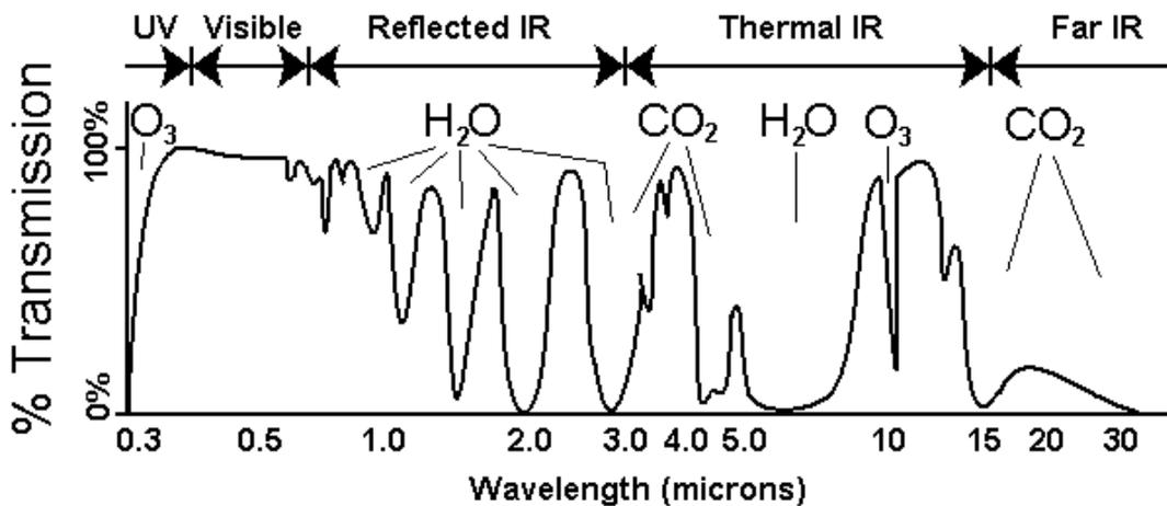
Figure 9: Wavelength versus Atmosphere Transmission Quality (Source: [www.rsc.org](http://www.rsc.org))
