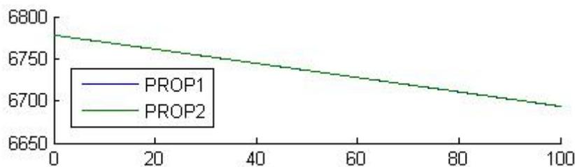
Figure 3: Change in semi-major axis due to atmospheric drag (km) over 100 solar days.
