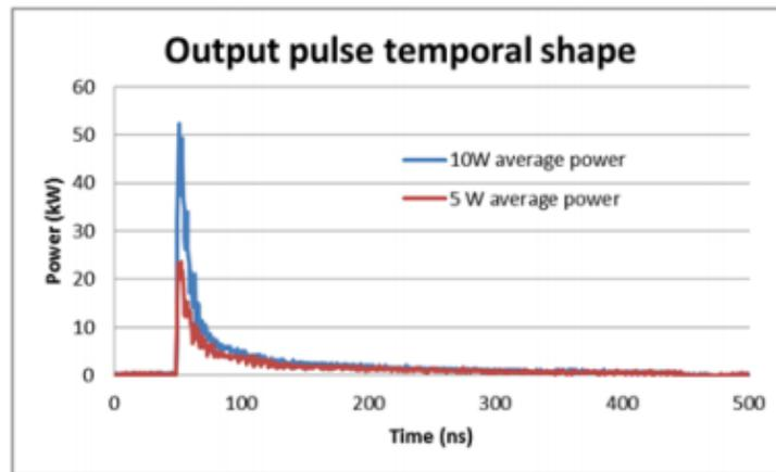
Figure 10: Typical pulse shape for optical amplifier (Source: [www.coractive.com](http://www.coractive.com))
