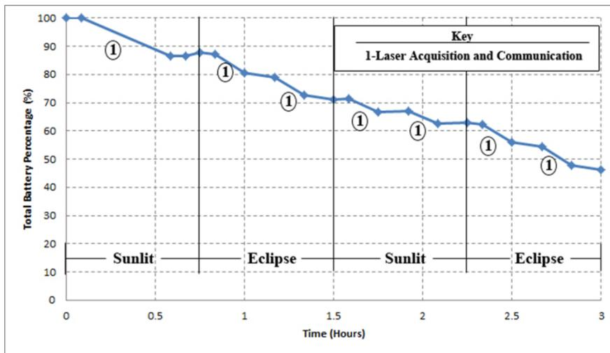
Figure 16: Expected Total Battery Percentage over 3 hours
