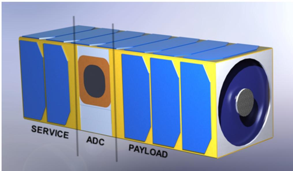
Figure 18: Layout of Subsystems within Structure
