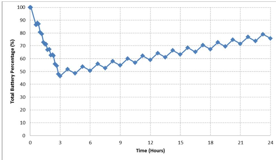
Figure 17: Expected Total Battery Percentage over 24 hours
